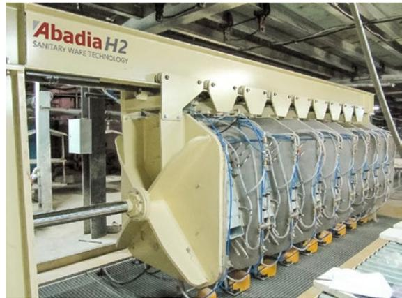
Abadia H2 high pressure casting plant designed for the production of wash basins. Its modification H2+ is also capable of making casting pedestals, squatting pans and shower trays.
